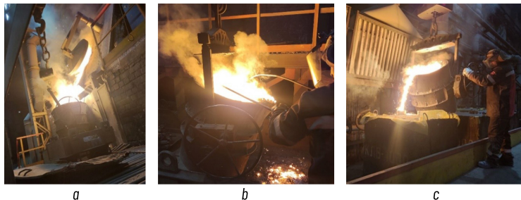
Fig. 5.3 Steel casting using a 3-tonne induction melting furnace from EGES (Turkey): a – pouring molten metal from the furnace into a ladle; b – skimming slag from the surface of the melt; c – filling molds during the casting stage
