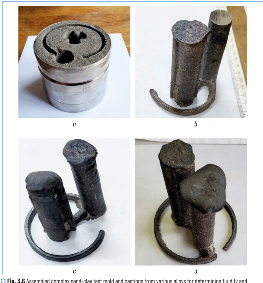
Fig. 3.6 Assembled complex sand-clay test mold and castings from various alloys for determining fluidity and mechanical properties: a – complex ring test mold; b – high-entropy alloy casting of the FeNiCrCuMn system ( \lambda = 105 mm); c – stainless steel casting GX10CrNiMn18-9-1 ( \lambda = 179 mm); d – gray cast iron ( \lambda = 265 mm)
