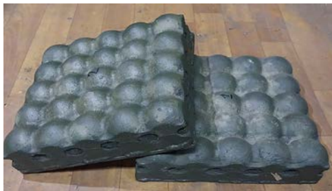
○ Fig. 4.27 Reinforced steel castings of the protective module, which were manufactured using the developed technology
