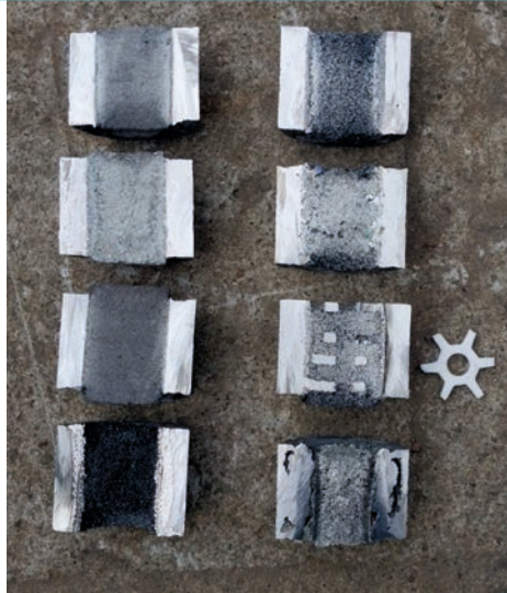
○ Fig. 4.19 Sections of cast samples with different fillers
