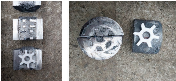
○ Fig. 4.20 Section of samples with quartz sand filler and membranes obtained by liquid-phase reinforcement
