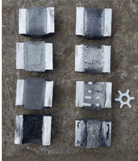
Fig. 4.19 Sections of cast samples with different fillers
