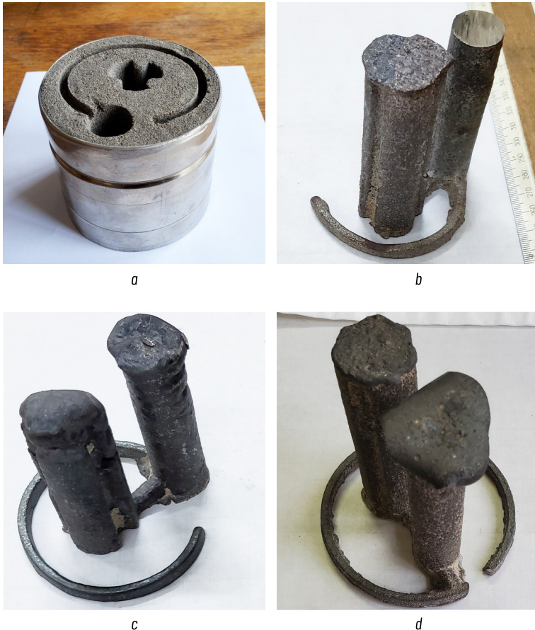
Fig. 3.6 Assembled complex sand-clay test mold and castings from various alloys for determining fluidity and mechanical properties: a – complex ring test mold; b – high-entropy alloy casting of the FeNiCrCuMn system ( \lambda = 105 mm); c – stainless steel casting GX10CrNiMn18-9-1 ( \lambda = 179 mm); d – gray cast iron ( \lambda = 265 mm)
