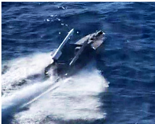
Fig. 3.4 "Magura V5" USV appearance with installed P-73 air-to-air missiles Source: [35]
