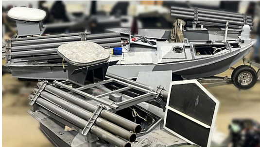
Fig. 3.6 "SeaBaby" USV appearance with guides for the use of 122-mm shells Source: [38]
