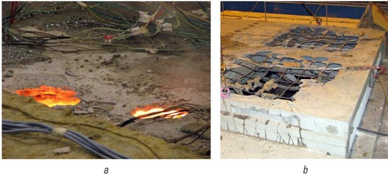
**Fig. 3.14** The nature of the destruction of the panel of the ribbed reinforced concrete slab during its fire tests: *a* – during the fire tests; *b* – after the fire tests
