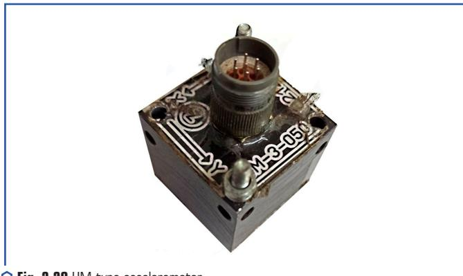
○ Fig. 2.20 UM-type accelerometer
