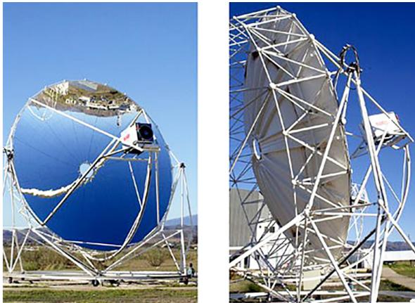
**Fig. 2.5** Solar concentrator from EuroDish
