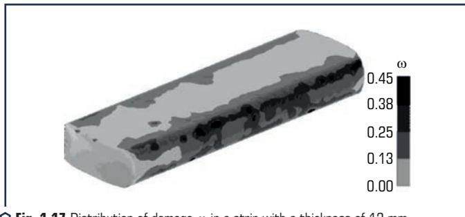
○ Fig. 1.17 Distribution of damage  $\omega$  in a strip with a thickness of 12 mm
