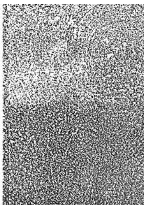
**Fig. 4.4** Macrostructure of the longitudinal section of a continuously cast ingot  $\varnothing 90$  mm from the B96Ts alloy: the upper part – without electromagnetic stirring; the lower one – with electromagnetic stirring of the alloy in the ingot
