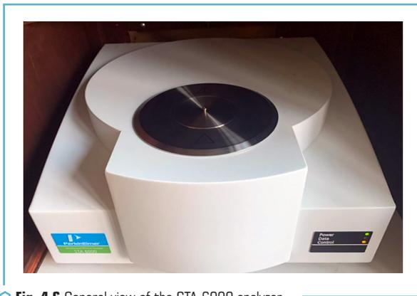
Fig. 4.6 General view of the STA-6000 analyzer
