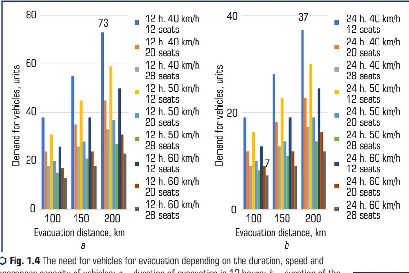
○ Fig. 1.4 The need for vehicles for evacuation depending on the duration, speed and passenger capacity of vehicles: *a* – duration of evacuation is 12 hours; *b* – duration of the evacuation is 24 hours (twice the time to evacuate, the number of evacuees is the same)
