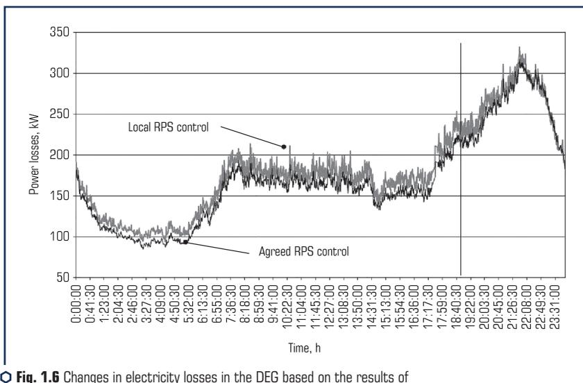
**Fig. 1.6** Changes in electricity losses in the DEG based on the results of the AUKRM-160 RPS operation at TS-557
