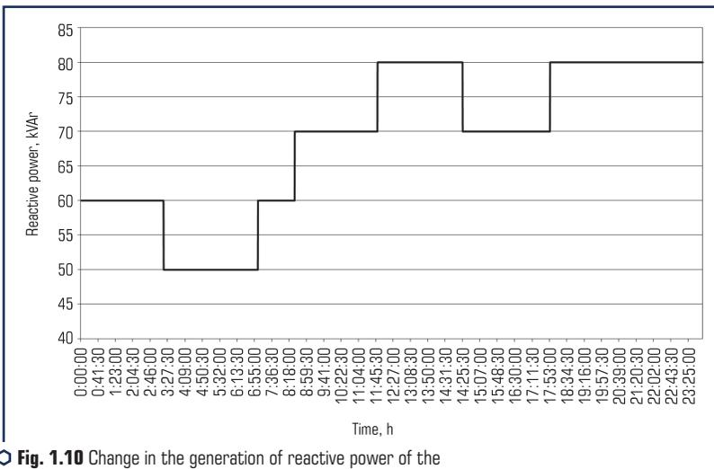
Fig. 1.10 Change in the generation of reactive power of the compensating plant installed at TS-496
