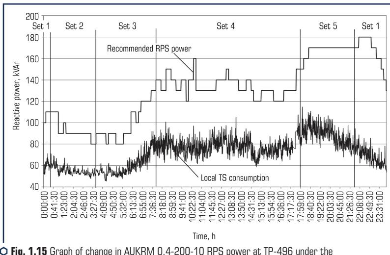
Fig. 1.15 Graph of change in AUKRM 0.4-200-10 RPS power at TP-496 under the influence of local ACS after optimization of its debugging parameters
