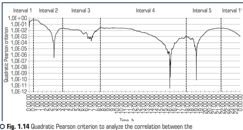
Fig. 1.14 Quadratic Pearson criterion to analyze the correlation between the sets  $Q_{opt}/Q_{REV}$  and  $Q_{REV}$  (logarithmic scale)
