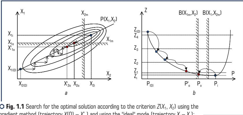
**Fig. 1.1** Search for the optimal solution according to the criterion  $Z(X_1, X_2)$  using the gradient method (trajectory  $X(0) - X^*_o$ ) and using the "ideal" mode (trajectory  $X_i - X_o$ ):
