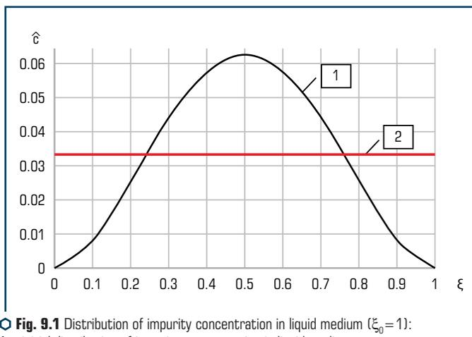
Fig. 9.1 Distribution of impurity concentration in liquid medium ( $\xi_0=1$ ):
