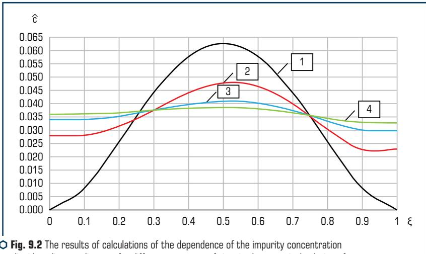
Fig. 9.2 The results of calculations of the dependence of the impurity concentration in a liquid medium on distance for different moments of time in the numerical solution of the problem: 1 –  $\tau=0$ ; 2 –  $\tau=0.03$ ; 3 –  $\tau=0.06$ ; 4 –  $\tau=0.09$
