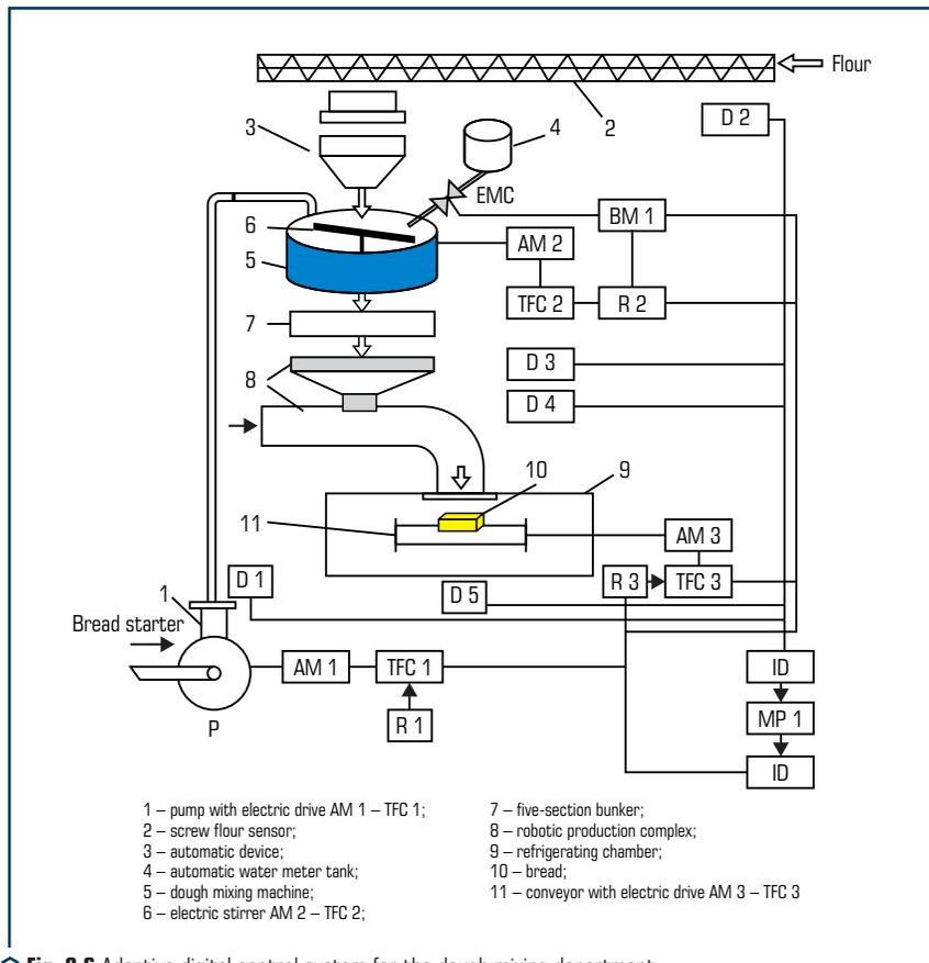
An analysis of the results of the functioning of the algorithm and structure of the adaptive automated control system (ACS) with monitoring of equipment performance (monitoring of product quality) allows us to conclude that the method of constructing adaptive ACS allows to synthesize fuzzy controllers for elementary operations of technological processes of bread production, taking into account the nonlinearity of objects of control project.
