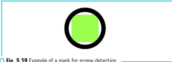
Fig. 5.19 Example of a mark for screw detection
