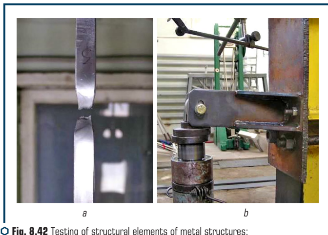
Fig. 8.42 Testing of structural elements of metal structures: a – tensile welded joint; b – bracket test
